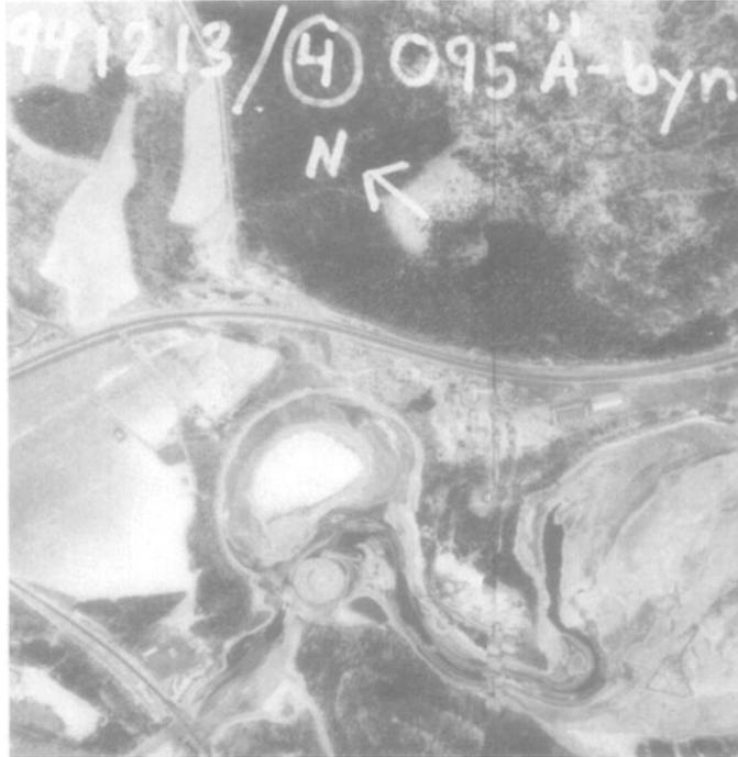
*Fig. 3 Overview of the rotating ice disc (diameter 79.8m) on the Pite River, 1994. The slightly oval shape of the ice disc indicates that the camera that took this high-altitude photograph was not exactly above the centre of the disc. (Courtesy of Akktu Stakki, Swedish Air Force.)*
