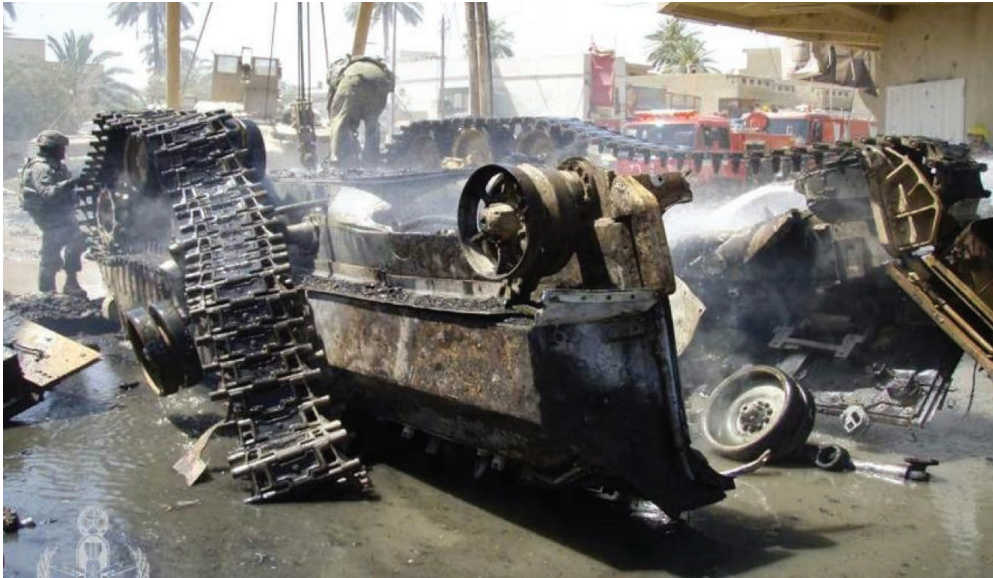
Figure 2.2 Bradley Fighting Vehicle Destroyed by a Deeply Buried IED
