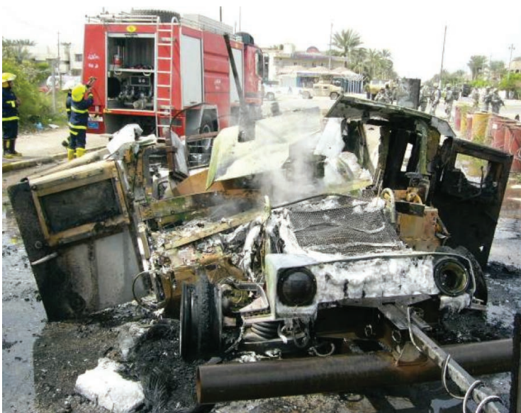
Figure 2.1 HMMWV Destroyed by EFP
