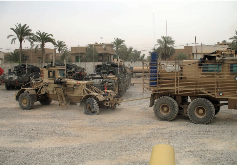
Figure 4.14 Battle-Damaged Husky Vehicle Mounted Mine Detection (VMMD) System
