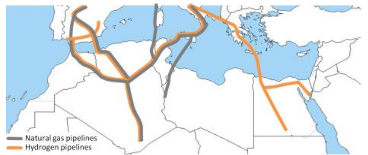
Figure 5. Natural gas infrastructure Europe - North Africa (left figure) and first outline for a hydrogen backbone infrastructure Europe-North Africa (figure above) An existing gas infrastructure from Algeria and Morocco could be converted to a hydrogen infrastructure (grey-orange lines). A “new” hydrogen transport pipeline must be realized from Italy to Greece, crossing the Mediterranean Sea to Egypt, which could eventually be extended to the Middle East (orange line).
