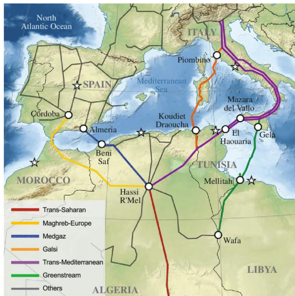
Figure 5. Natural gas infrastructure Europe - North Africa (left figure) and first outline for a hydrogen backbone infrastructure Europe-North Africa (figure above) An existing gas infrastructure from Algeria and Morocco could be converted to a hydrogen infrastructure (grey-orange lines). A “new” hydrogen transport pipeline must be realized from Italy to Greece, crossing the Mediterranean Sea to Egypt, which could eventually be extended to the Middle East (orange line).
